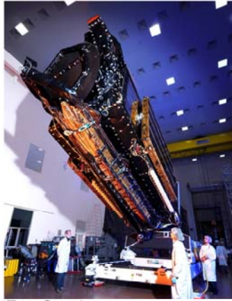
TerreStar-1 18-meter antenna reflector (courtesy Space Systems/Loral)
